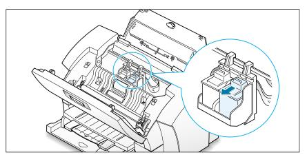
7. Lift the cartridge up and out of the cartridge holder.
